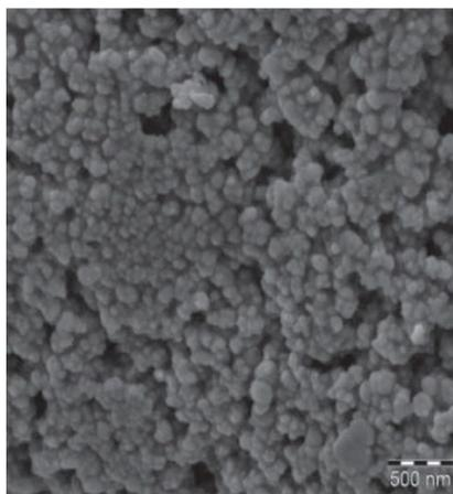
Figure 4 - SEM image of zinc sulfide (ZnS) nanoparticles synthesized by the thermolysis of the precursor Zinc (II) bis (N,N-diallyl dithiocarbamate) in hexadecylamine [2].
