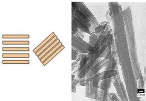
Figure 3: SEM and schematic image of nanoclay sheets [1].
