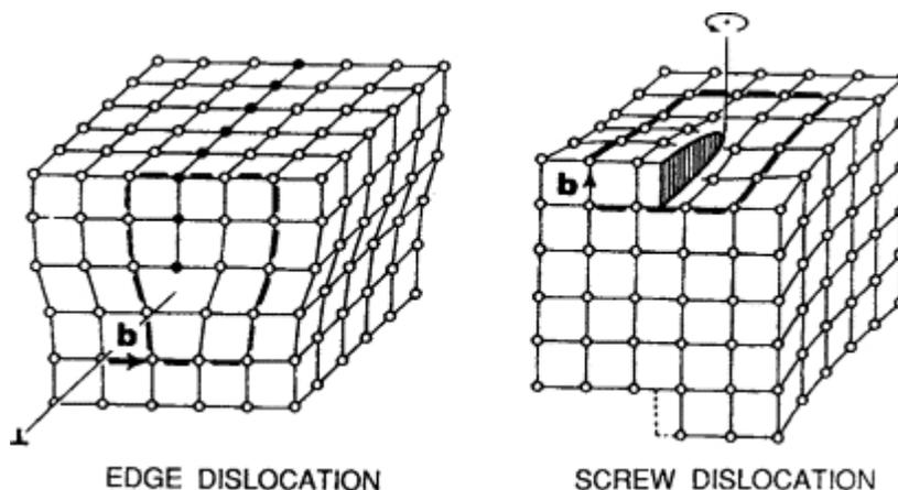
Figure 8: Representation of edge and screw dislocations.
