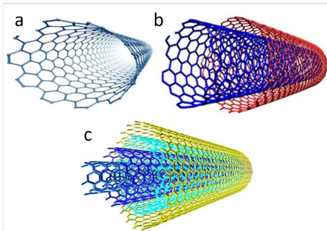
Figure 2: Types of carbon nanotubes based on the number of walls: (a) Single-walled carbon nanotubes, (b) Double-walled carbon nanotubes, and (c) Multi-walled carbon nanotubes [2].
