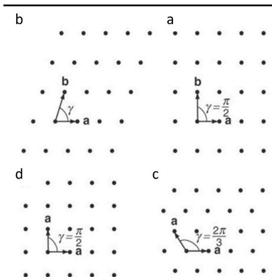
Figure 2: Four different two-dimensional crystal systems: (a) rectangular, (b) oblique, (c) hexagonal, (d) square. [1].
