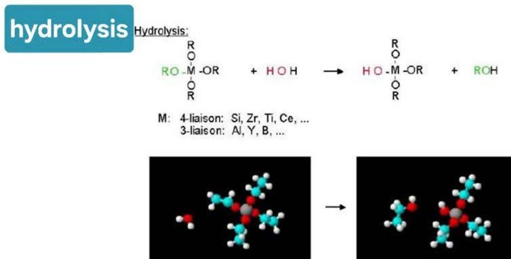
Figure 3 - Overview of the hydrolysis reaction for a metal alkoxide
