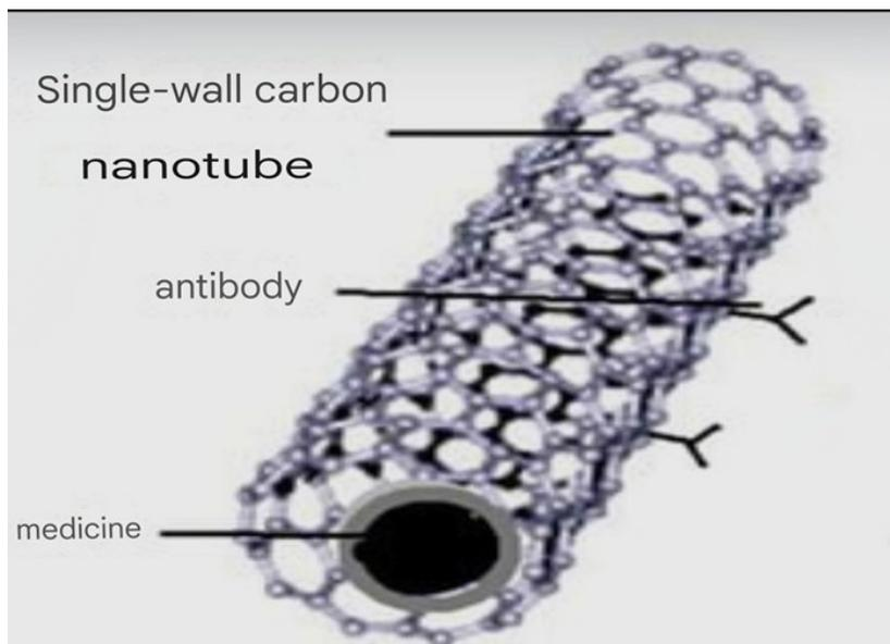
Figure 5: Drug loading inside the hollow core of a single-walled carbon nanotube for targeted drug delivery [3].
