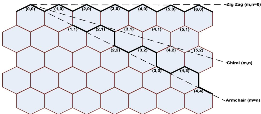
Figure 4: A graphene sheet with three different points, each corresponding to a different type of carbon nanotube.
