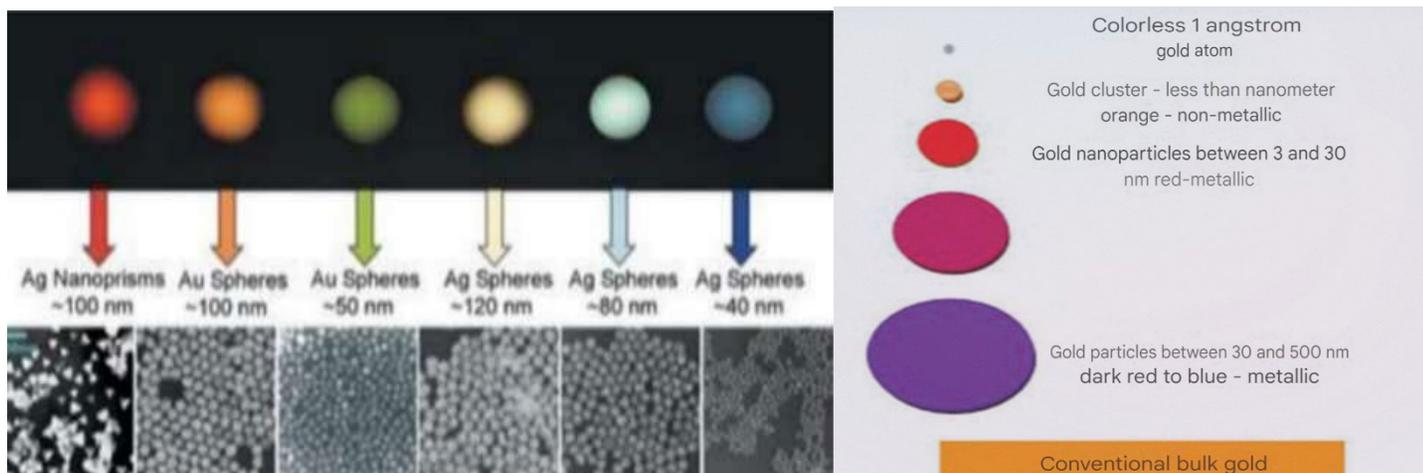
Figure 3: (a) Colors of gold nanoparticles at different sizes, (b) Colors of gold and silver nanoparticles with different shapes and sizes
