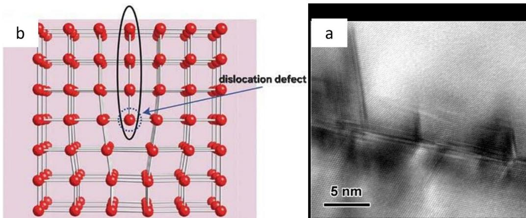
Figure 2 - (a) TEM image and (b) schematic representation of a dislocation defect [1].
