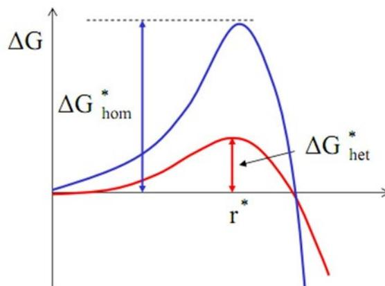
Figure 5: Comparison between free energy in homogeneous (blue) and heterogeneous (red) nucleation and growth [1].
