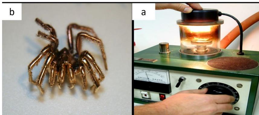
Figure 9 - (a) A schematic of the sputtering device for SEM sample coating. (b) A gold-coated spider prepared for SEM analysis.
