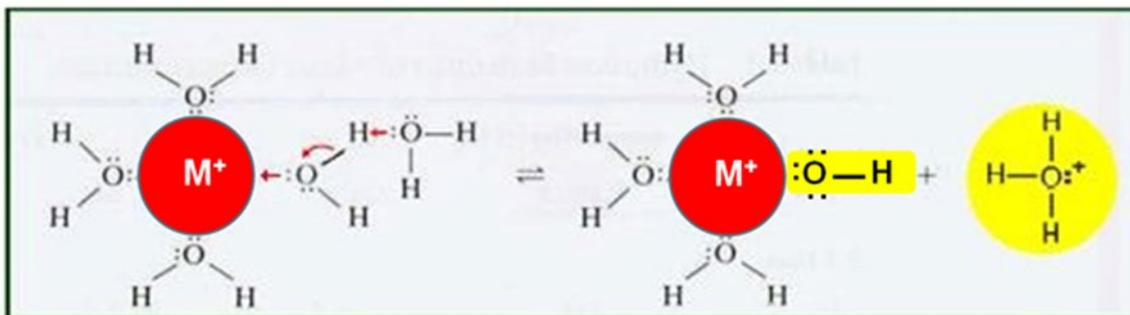
Figure 3 - A schematic representation of the hydrolysis process of metal cations.\*\*
