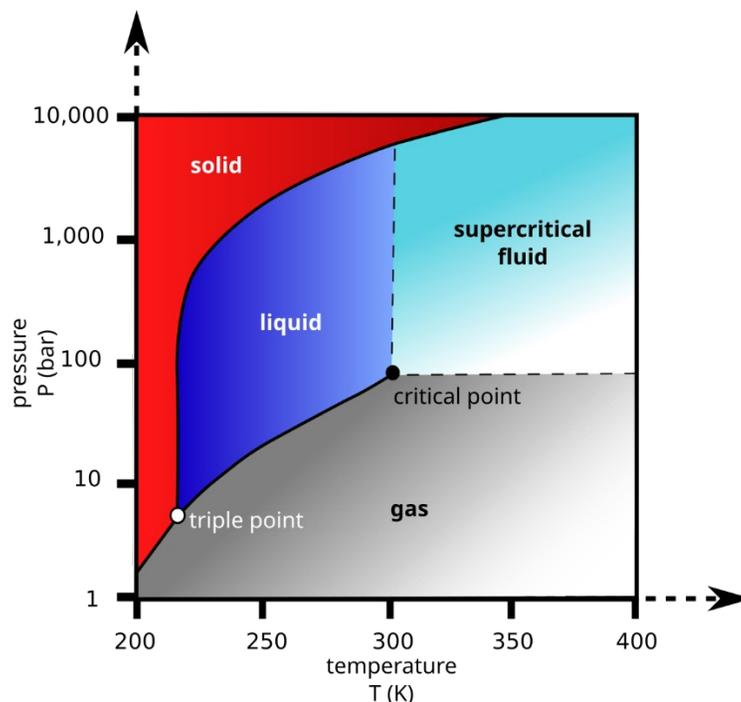
Figure 7 - Pressure-temperature phase diagram for reaching critical conditions.
