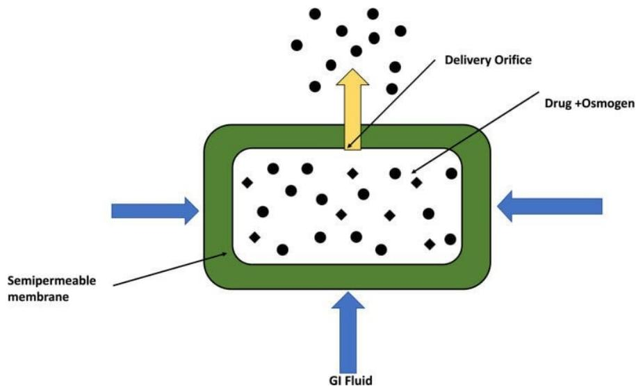
Figure 2 - Schematic of the drug release mechanism using simple osmotic pumps [2].
