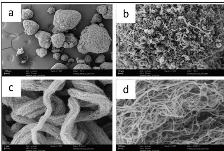
Figure 2: SEM image of carbon nanotube aggregates at different magnifications (from (a) to (t) magnification increases) [2].
