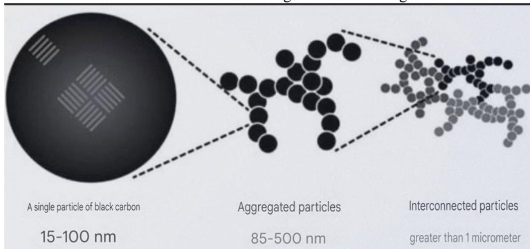
Figure 9: Diagram showing different forms of carbon black with their size ranges.
