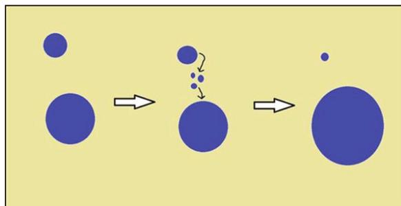
Figure 4 - A schematic of the Ostwald ripening process, where smaller particles dissolve, and larger ones grow.
