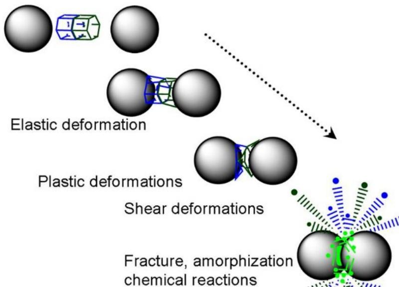
Figure 2 - The three main stages of the initial powder crushing and size reduction process.
