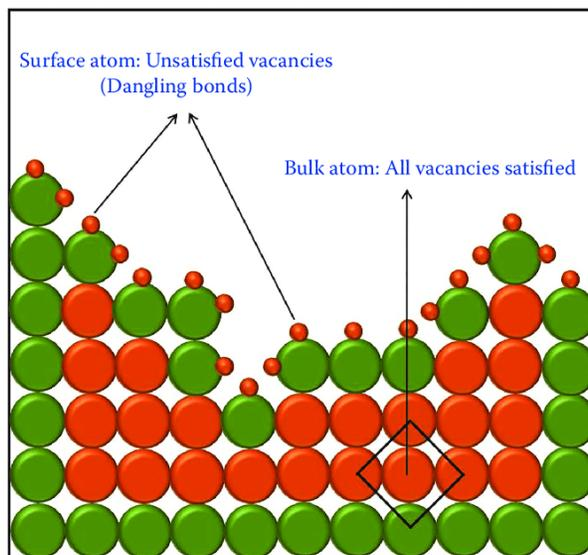
Figure 4: Comparison between surface atoms and bulk atoms.
