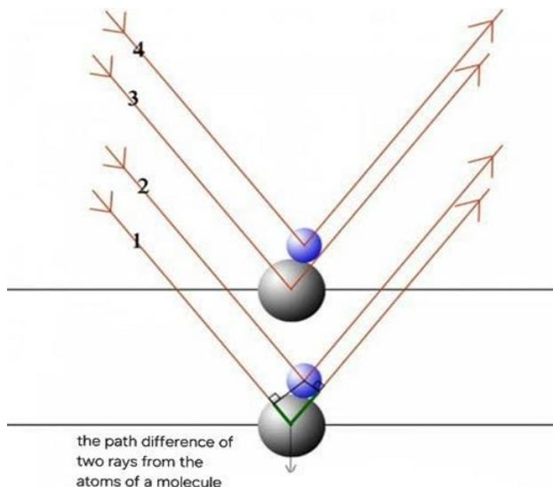
Figure 5 shows the impact of atomic arrangement on the intensity of reflected X-rays. The green section represents the path difference between X-rays 1 and 2.
