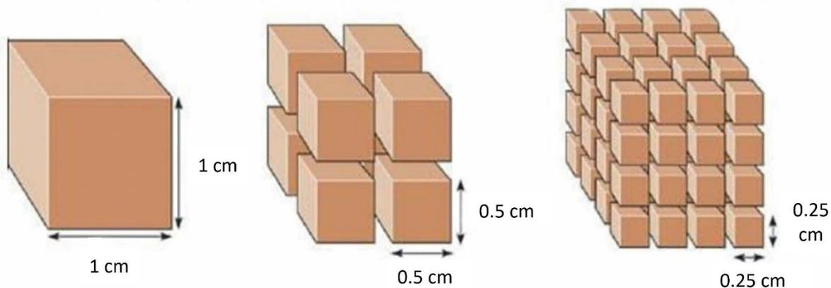
Figure 3: Each step of cutting results in eight smaller cubes.
