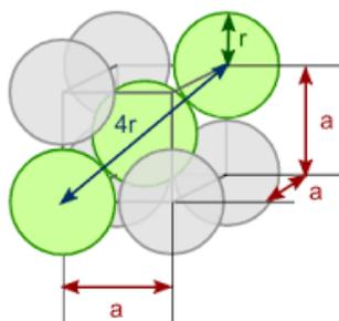
Figure 9: Showing the Packed vector and the relationship between the cube edge length and atomic radius in the body-centered cubic lattice.
