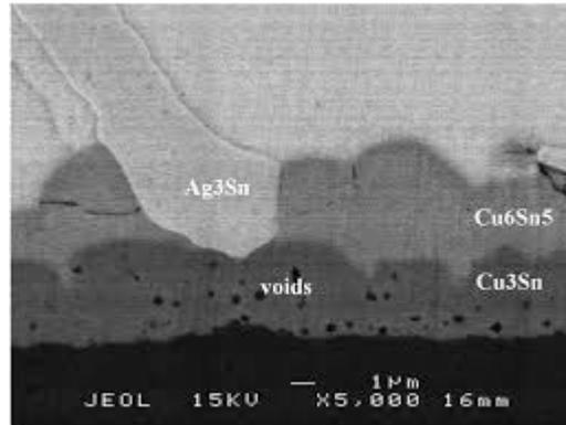
Figure 10: Representation of voids (three-dimensional defect) in an SEM image.
