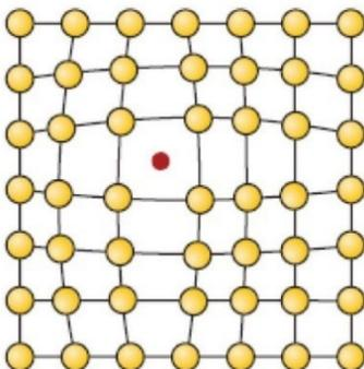
Figure 3: Representation of an interstitial atom in a crystal structure.
