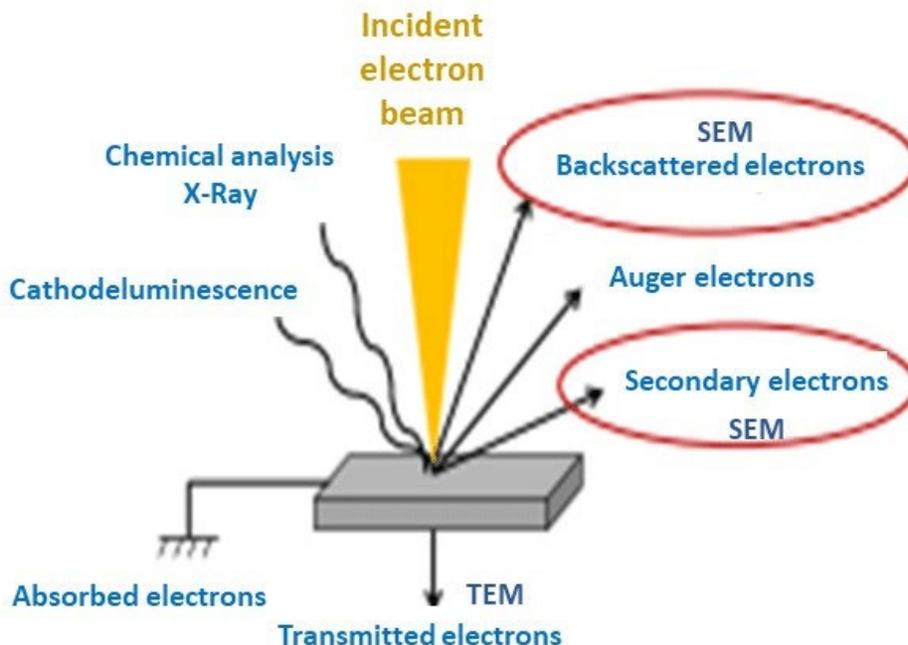
Figure 5 - Electron-Sample Interaction
