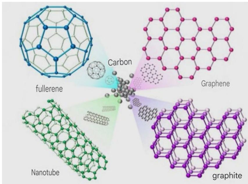
Figure 9: Geometric shapes of different carbon allotropes [6].
