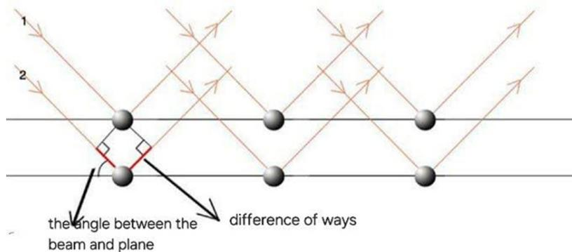
Figure 4 shows X-ray diffraction by a regular array of atoms. The red section represents the path difference between the two rays.
