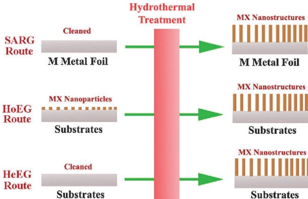
Figure 6: A schematic of the types of substrate-based hydrothermal methods.
