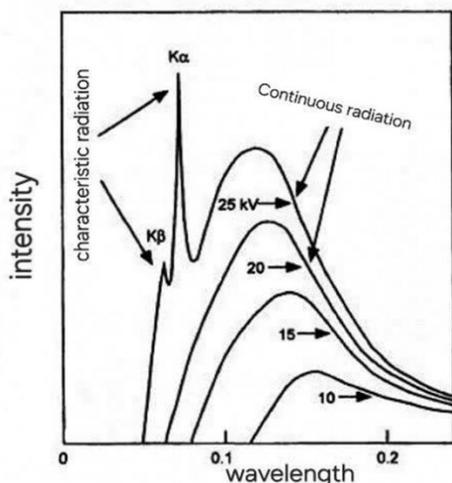
Figure 7 the radiation intensity spectrum of a target bombarded by electron beams as a function of wavelength.
