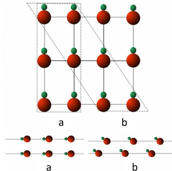
Figure 2 - Different interplanar spacing and the different arrangement of atoms in two planes of a crystal.
