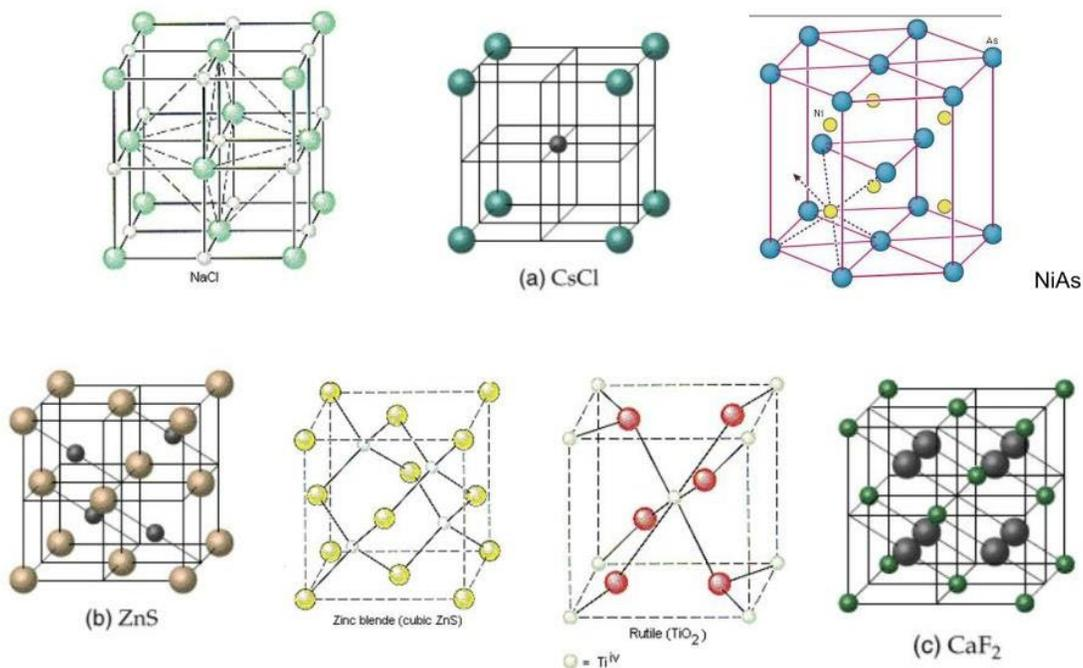
Figure 5: Well-known crystalline structures of ceramics (non-Bravais lattices).
