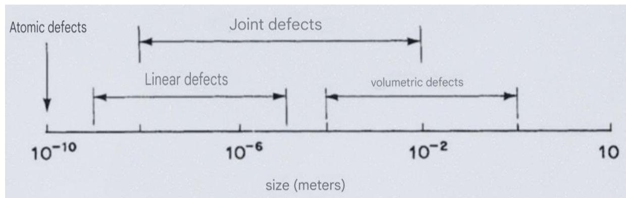
Figure 1: Various defects in a crystal and their size ranges.
