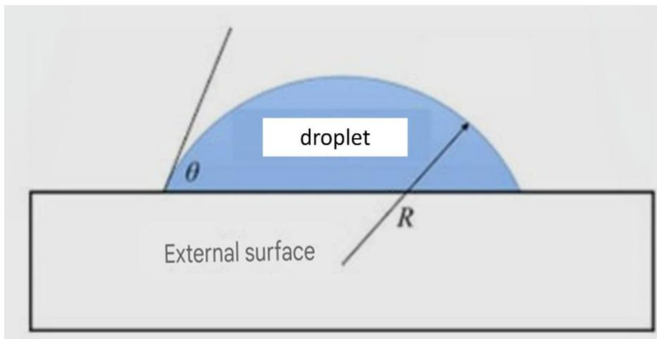
Figure 4: Formation of a nucleus on the external surface and its radius [2].
