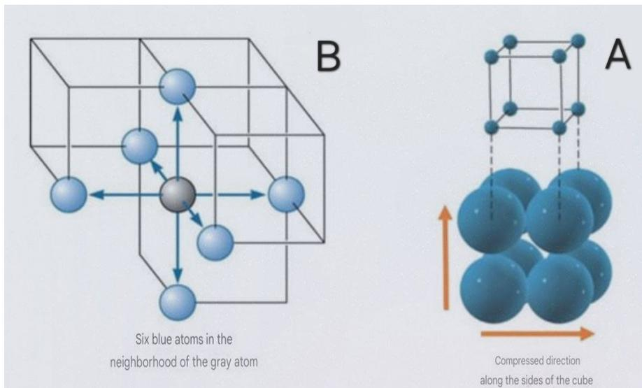
Figure 7 - Representation of a) Packed vector and b) coordination number in a simple cubic lattice
