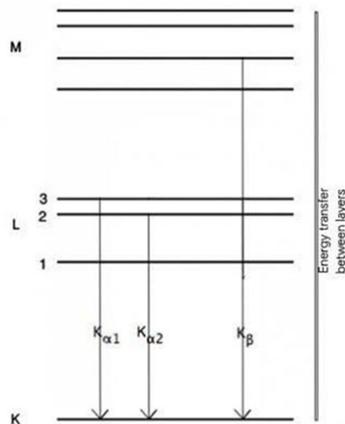
Figure 8 the energy levels of an atom and the associated transitions.
