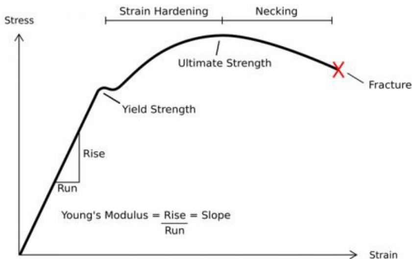
Figure 3: Stress-strain curve for materials, showing the direct relationship between stress and strain in the linear region.
