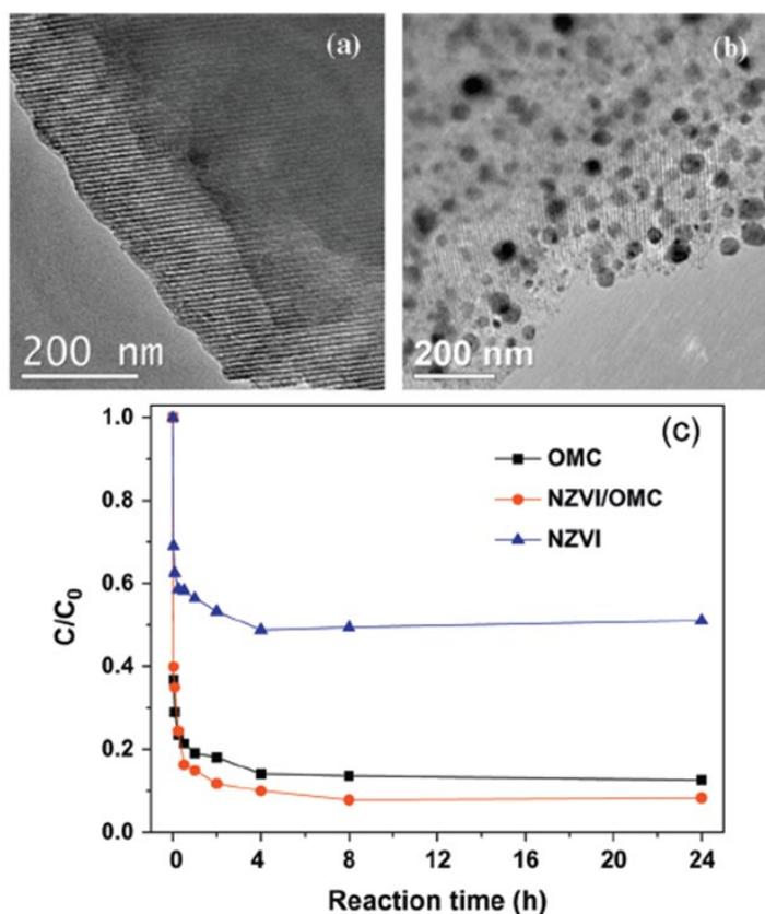
Figure 2. a) Transmission electron microscope image of mesoporous carbon and b) composite of mesoporous carbon and zero-valent iron nanoparticles c) ratio of pollutant concentration to initial concentration over time for each of the adsorbents
