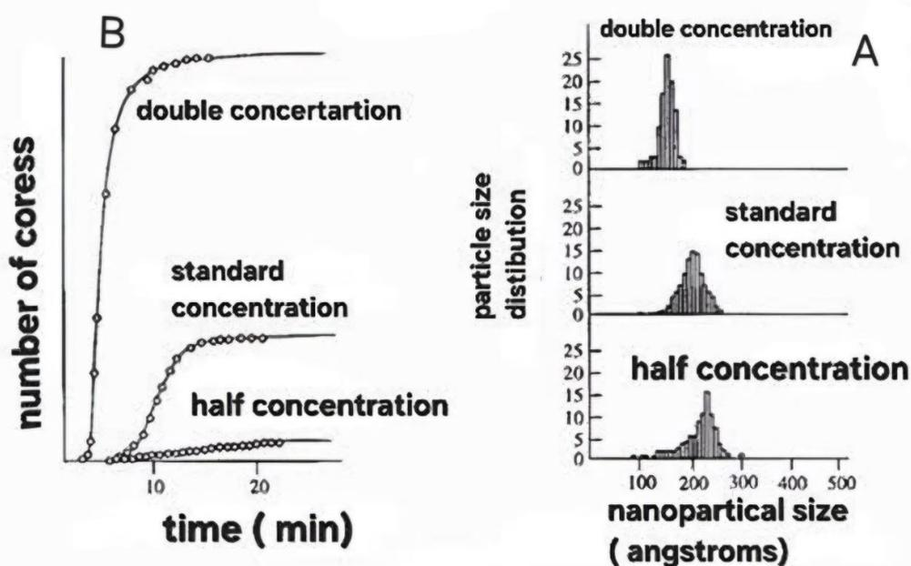
Figure 2: Effect of metal precursor concentration on (a) the number of nuclei formed at different times and (b) size distribution of metal nanoparticles synthesized via the chemical reduction method.
