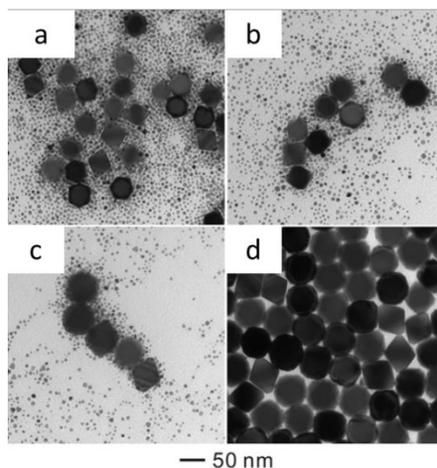
Figure 5 - TEM images showing Ostwald ripening in palladium nanoparticles dissolved in formaldehyde at different time intervals: (a) 6 hours, (b) 24 hours, (c) 48 hours, and (d) 72 hours [2].
