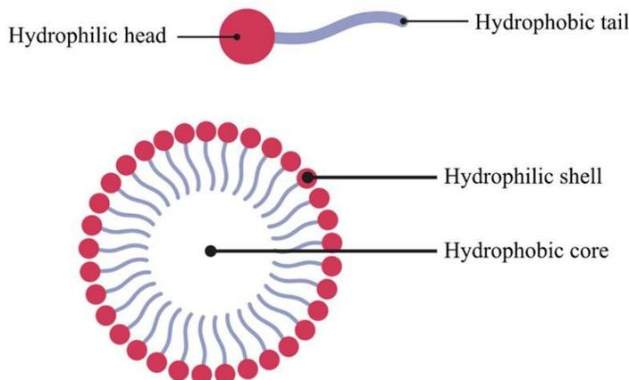
Figure 4 - Schematic showing the orientation of surfactants in a solution.
