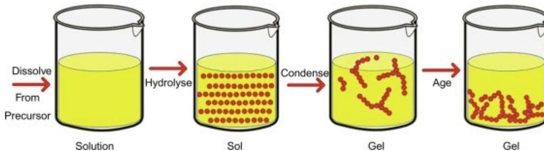
Figure 2 - Overview of all stages in the sol-gel process.
