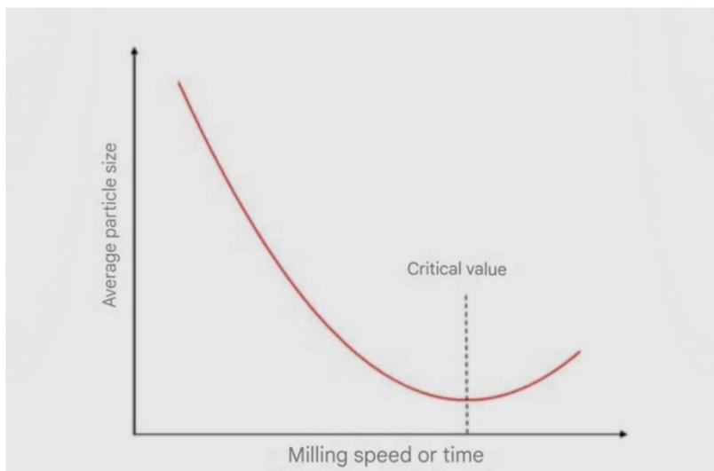
Figure 5 - Curve of average particle size variation as a function of milling speed or time.
