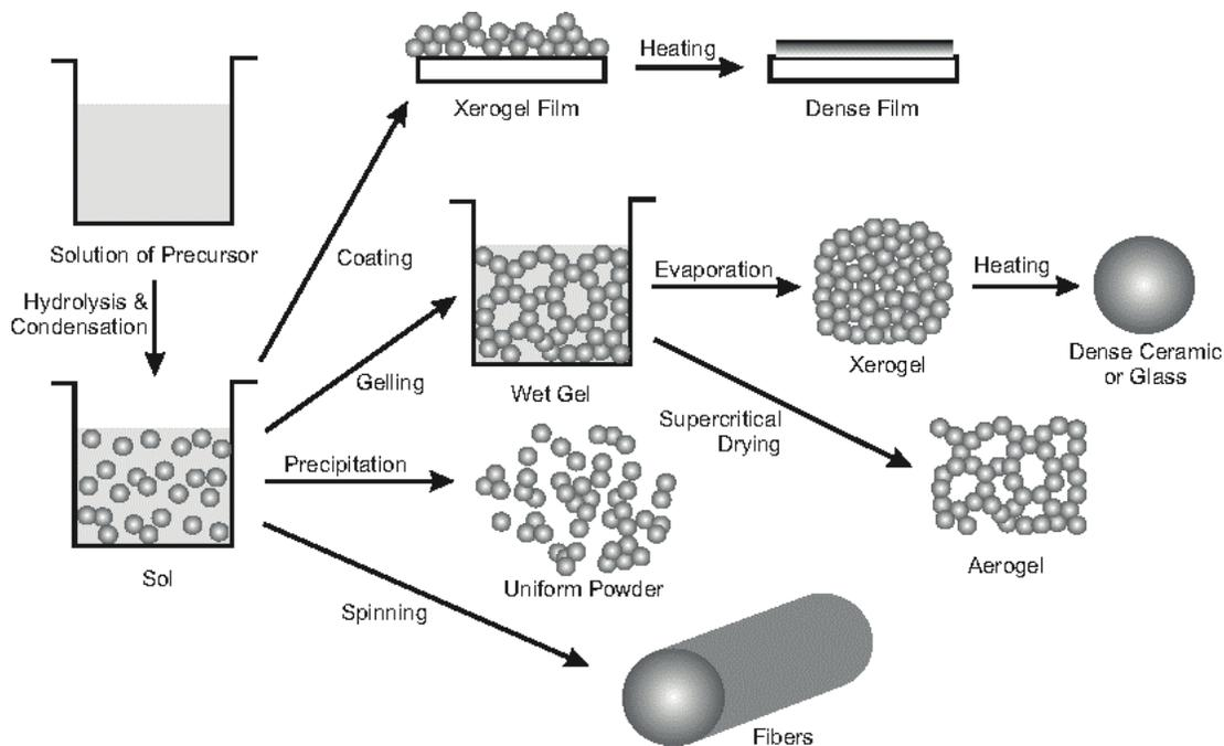
Figure 9 - Types of processes that can be performed in the sol-gel method and the products resulting from each process.
