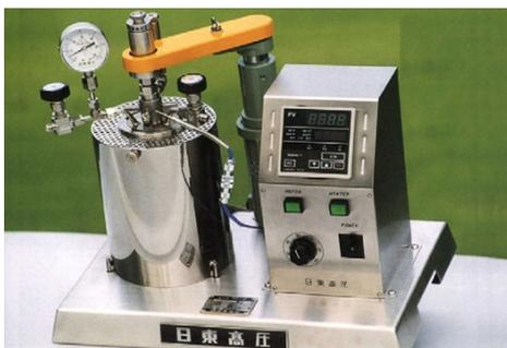
Figure 1 - An image of the hydrothermal device used for nanomaterial synthesis.
