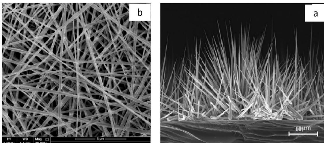
Figure 8: Images of one-dimensional nanostructures: (a) Zinc oxide nanowires, (b) PVP nanofibers.
