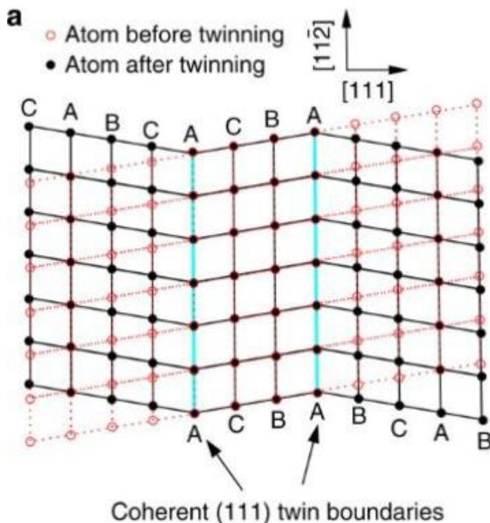
Figure 9: Representation of a twin boundary in a crystal, showing mirror symmetry on both sides.
