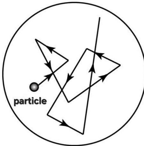
Figure 1 - Schematic representation of the Brownian motion of a particle in a fluid.
