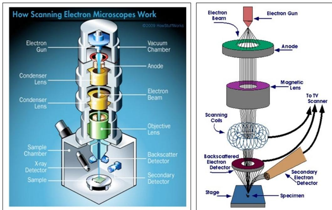
Figure 1 - Schematic of a Scanning Electron Microscope (SEM)
