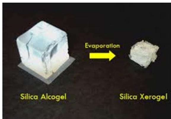
Figure 6 - Simple evaporation drying and the creation of xerogel.
