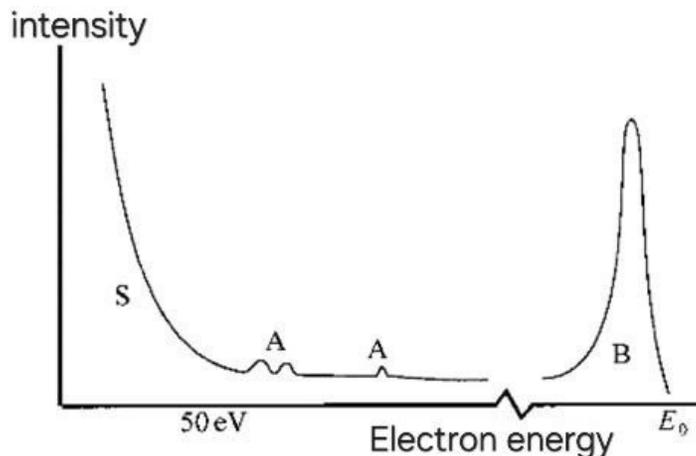
Figure 6 - Electron Spectrum Showing the Relative Abundance of Secondary Electrons (SE), Auger Electrons (A), and Backscattered Electrons (BSE) as a Function of Electron Energy
