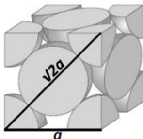
Figure 11: Showing the Packed vectors and the relationship between the cube edge length and atomic radius in the face-centered cubic lattice.
