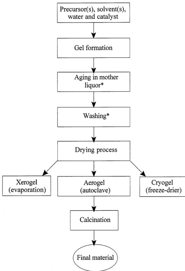
Figure 5 - Various stages of the sol-gel process and the aging stage.
