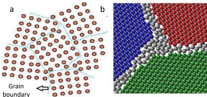
Figure 5: a) Grain boundaries as disordered regions separating grains in a polycrystalline material. b) Disordered arrangement at grain boundaries.
