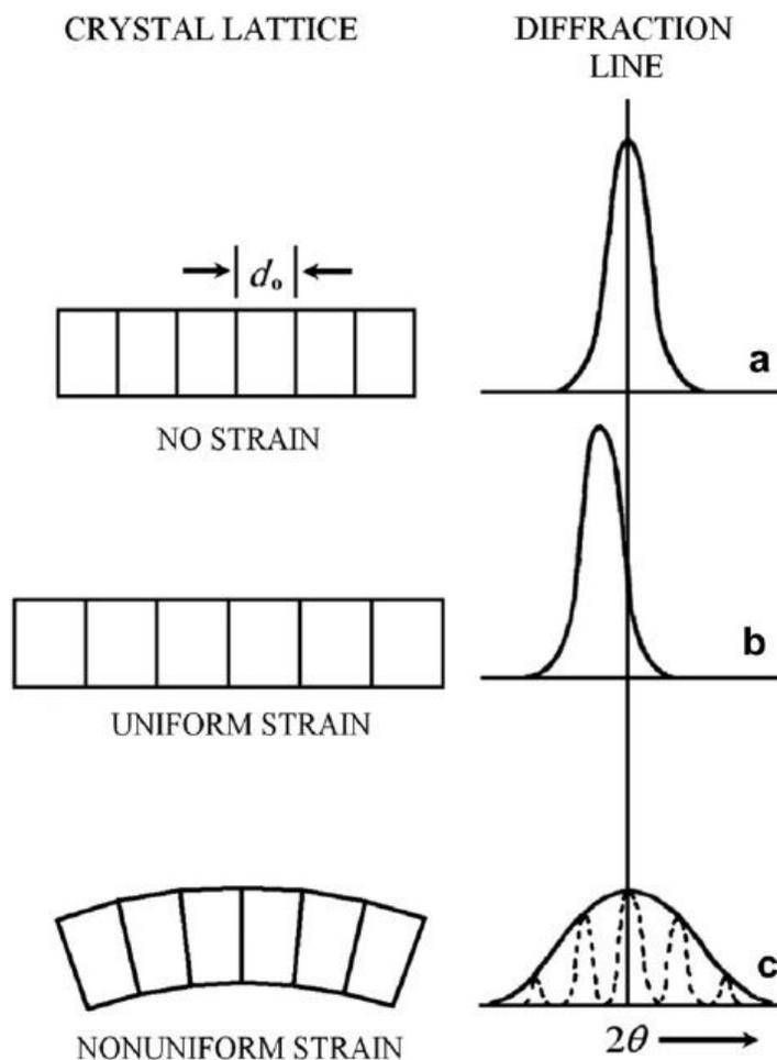
Figure 4: The effect of lattice strain on the position and width of the diffraction line.
