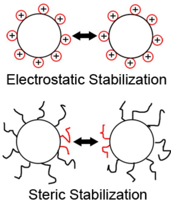
Figure 6 - A schematic of stabilization methods for preventing nanoparticle agglomeration.
