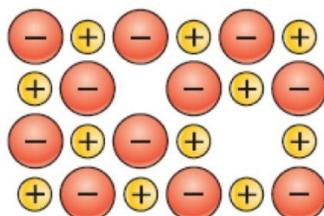
Figure 6: Representation of a Schottky defect.
