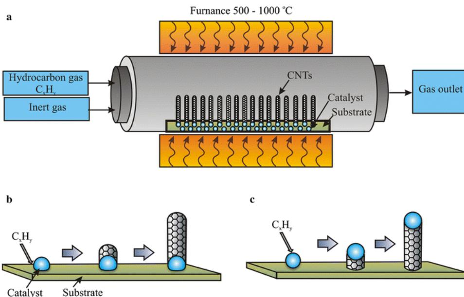
Figure 6: (a) A schematic of the Chemical Vapor Deposition process for synthesizing carbon nanotubes, (b) and (c) mechanisms for nanotube growth [4].
