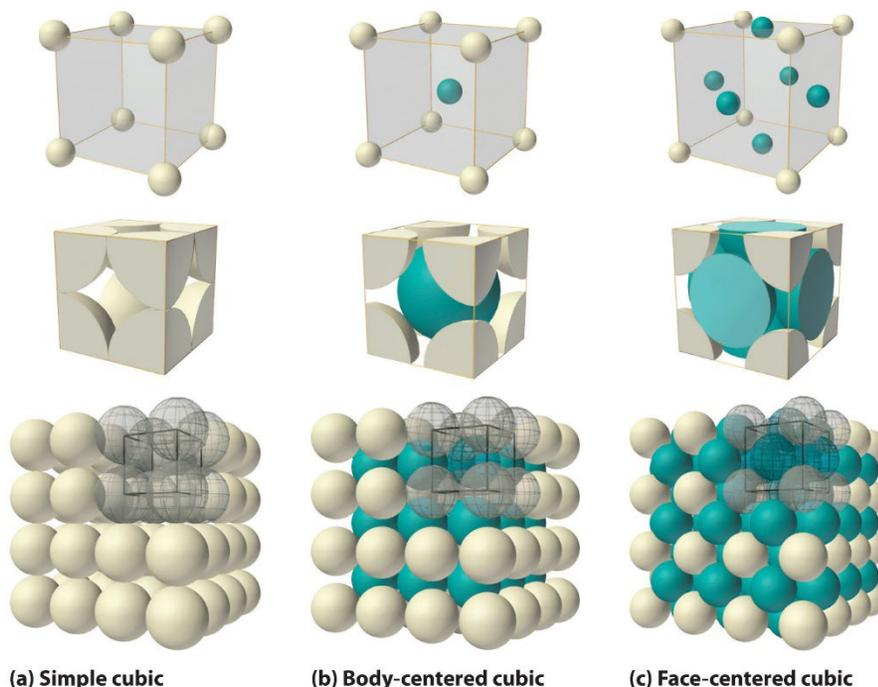
Figure 6: Schematic representation of the three cubic lattices: a) simple cubic, b) body-centered cubic, and c) face-centered cubic.
