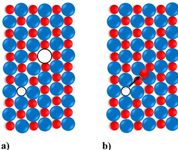
Figure 7: Representation of both Schottky(a) and Frenkel(b) defects occurring together in an ionic compound.
