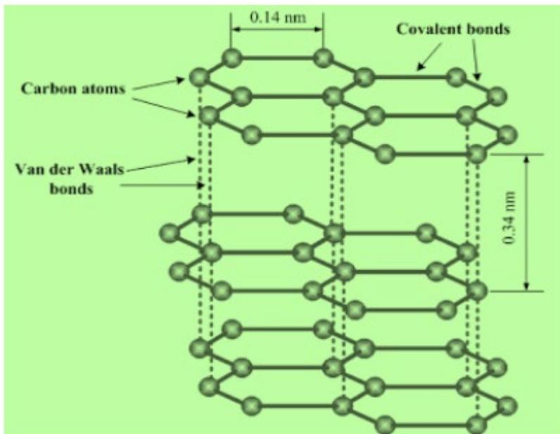
Figure 7: Diagram showing the layered structure of graphite, the type of bonds, and how the layers are arranged.
