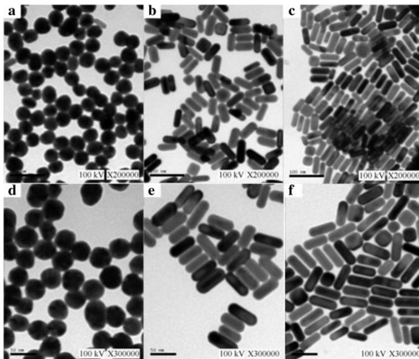
Figure 6: Images of nanoparticles with different shapes as zero-dimensional nanostructures.
