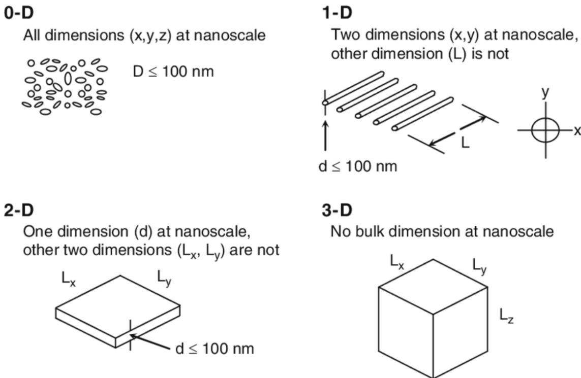
Figure 5: Types of nanostructures based on the number of free dimensions.
