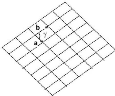
Figure 1: Defining a two-dimensional system with two vectors and the angle between them.
