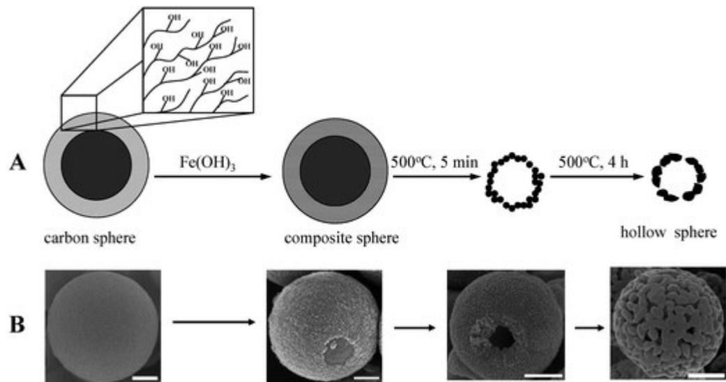
Figure 5 - (a) A schematic of the synthesis of iron oxide nanocages, and (b) scanning electron microscope (SEM) images of the product at each stage.
