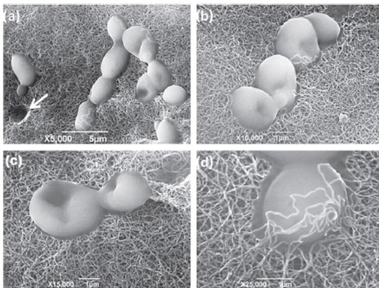
Figure 4. Scanning electron microscope image of nanotube/ceramic composite filter
