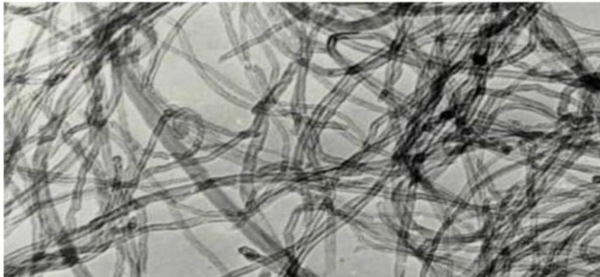
Figure 7: TEM image of carbon nanotubes synthesized by the CVD method [5].
