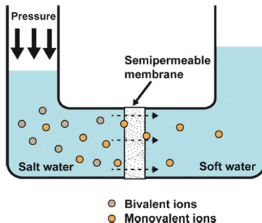
Figure3: The process of water hardness reduction using nanofiltration
