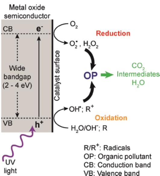
Figure 2. Photocatalytic treatment process [8]
