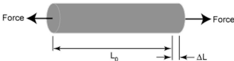
Figure 2: Deformation of a material due to applied stress.
