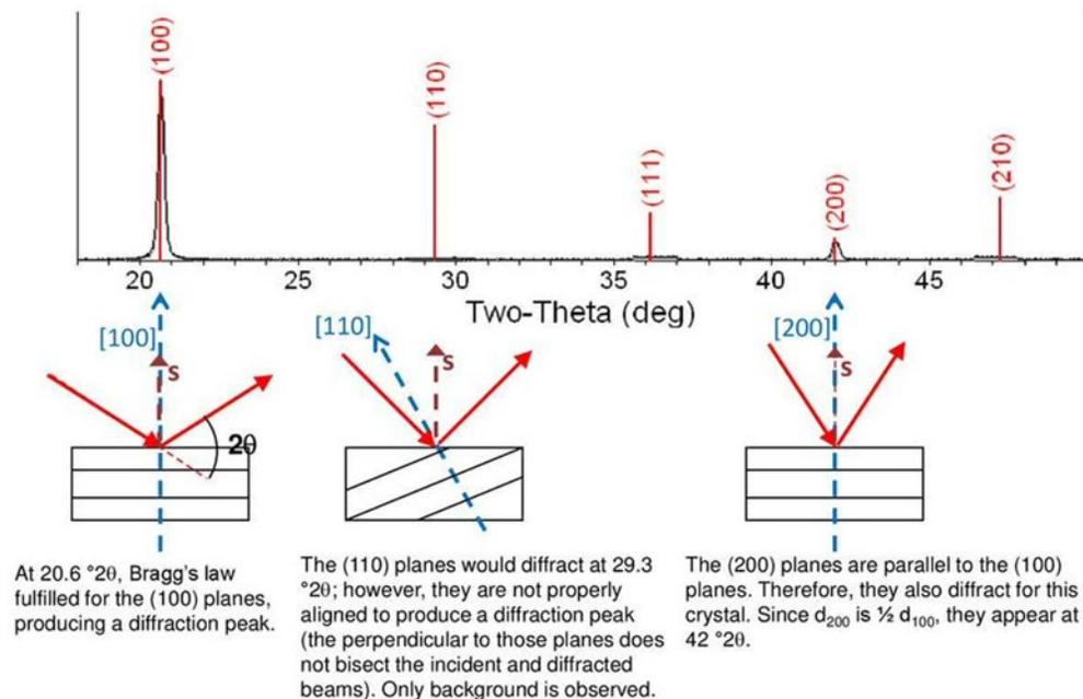
Figure 1: A schematic showing the effect of the crystal orientation on the diffraction peaks observed in the X-ray diffraction pattern of a single crystal.
