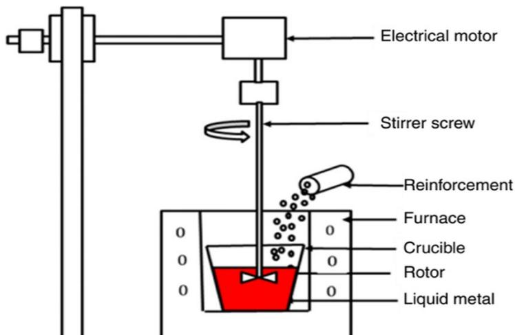
Figure 6: Production of Metal Matrix Nanocomposites via Stir Casting
