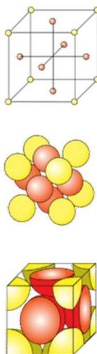
Figure 10: Schematic representation of a face-centered cubic lattice.
