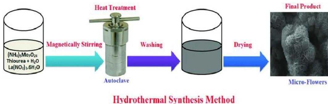
Figure 2 - Schematic of the hydrothermal process for synthesizing  $\text{MoS}_2$  nanostructures.
