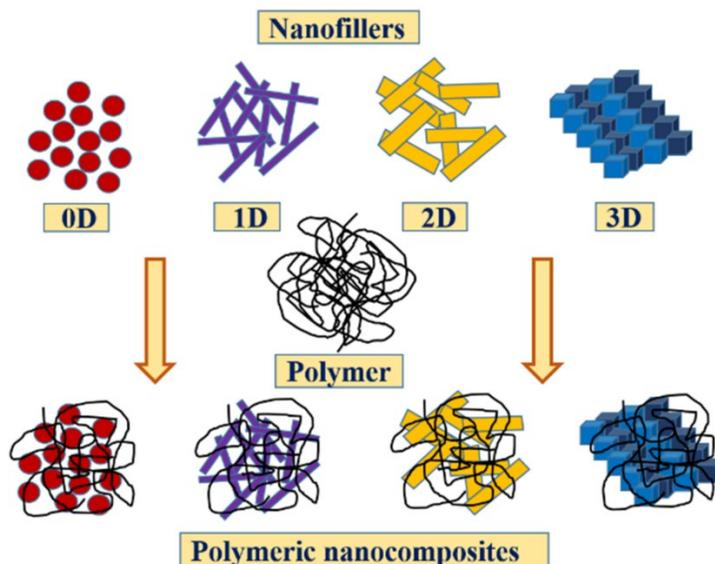
Figure 1: different kind of nanomaterial can be used as nanofillers in nanocomposites
