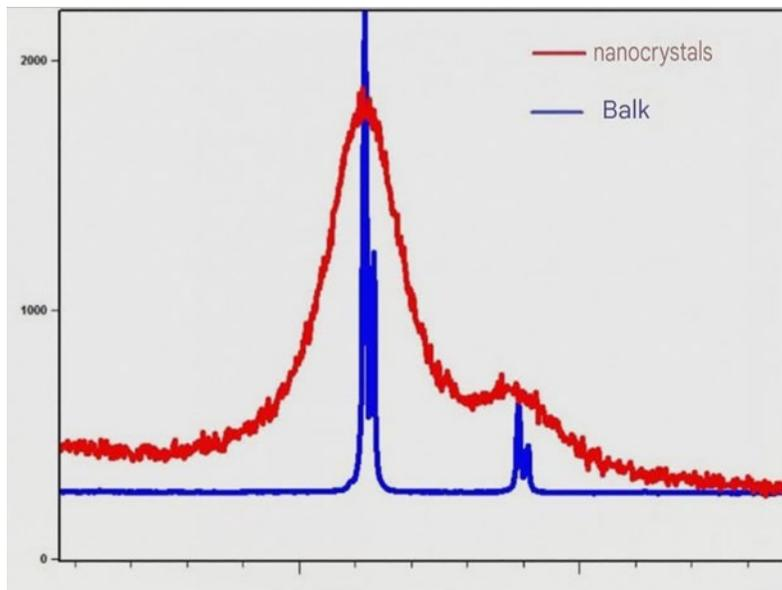
Figure 2: X-ray diffraction patterns of cerium oxide in bulk and nanoparticle forms.
