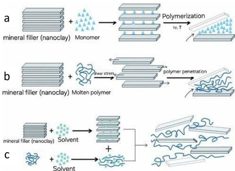
Figure 5: Schematic of methods for producing polymeric nanocomposites with nanoclay [3].
