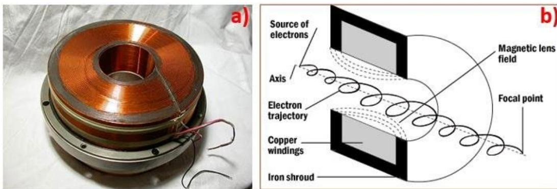
Figure 4 - (a) Schematic of How an Electromagnetic Lens Works, and (b) Real Image of an Electromagnetic Len
