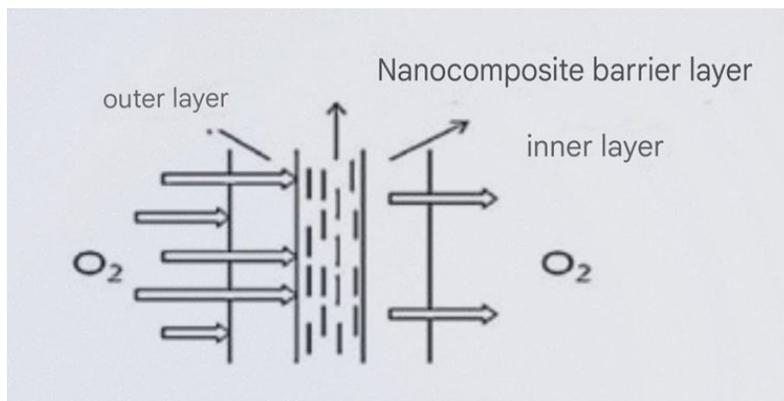
Figure 8: Use of nanoclay as a barrier to prevent oxygen from entering food packaging [6].
