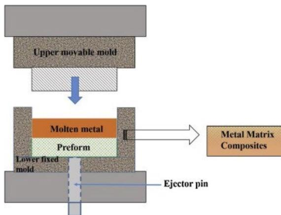
Figure 7: Schematic of the Melt Infiltration Process for Metal Matrix Nanocomposites
