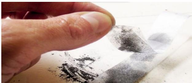
Figure 10: The mechanical exfoliation method for synthesizing graphene from high-crystalline graphite.
