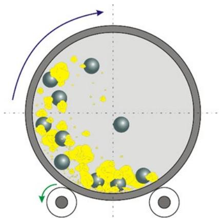
Figure 1 - A simple illustration of the inside of a ball mill.
