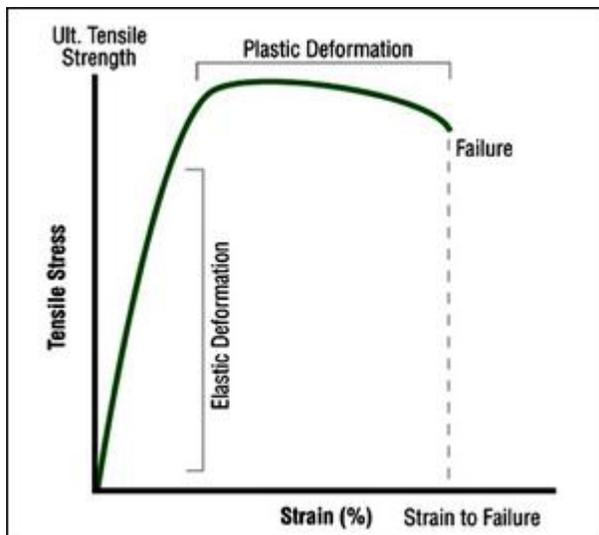
Figure 4: Stress-strain curve obtained from a tensile test of a sample.
