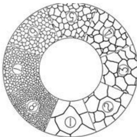
Figure 7: The eight stages of grain refinement due to the application of mechanical forces on a material. As the process progresses, the number of grains increases while their size decreases.
