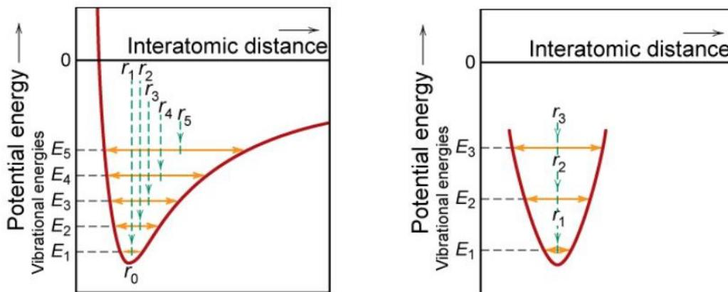
Figure 2: Potential energy diagrams (vertical axis) as a function of interatomic distance (horizontal axis) at various vibrational energies of a material (due to increased temperature). a) For a material with symmetric potential wells, b) For a material with asymmetric potential wells [1].
