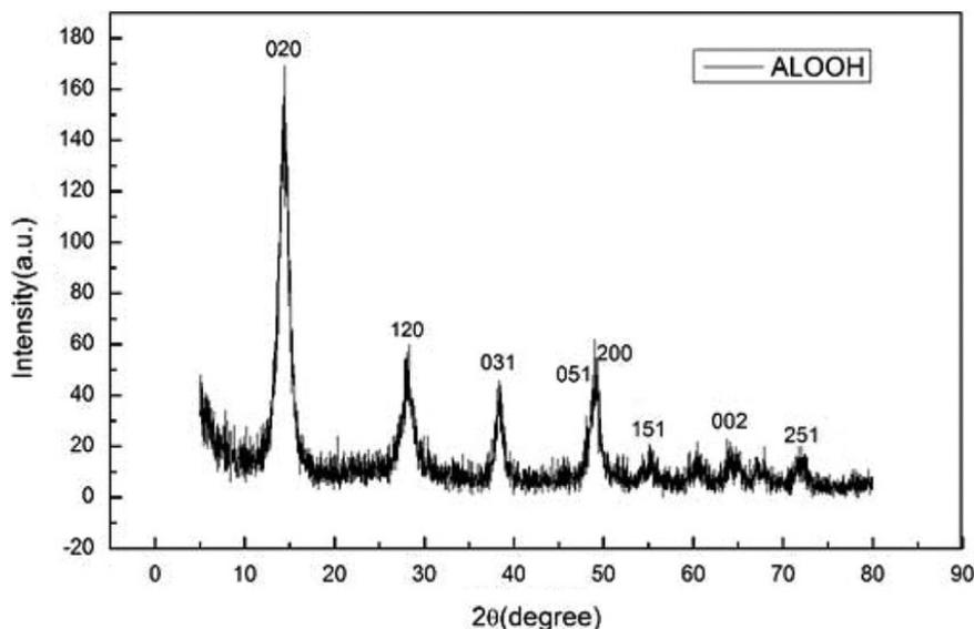
Figure 1 - Example of Data Recorded from Powder Diffraction
