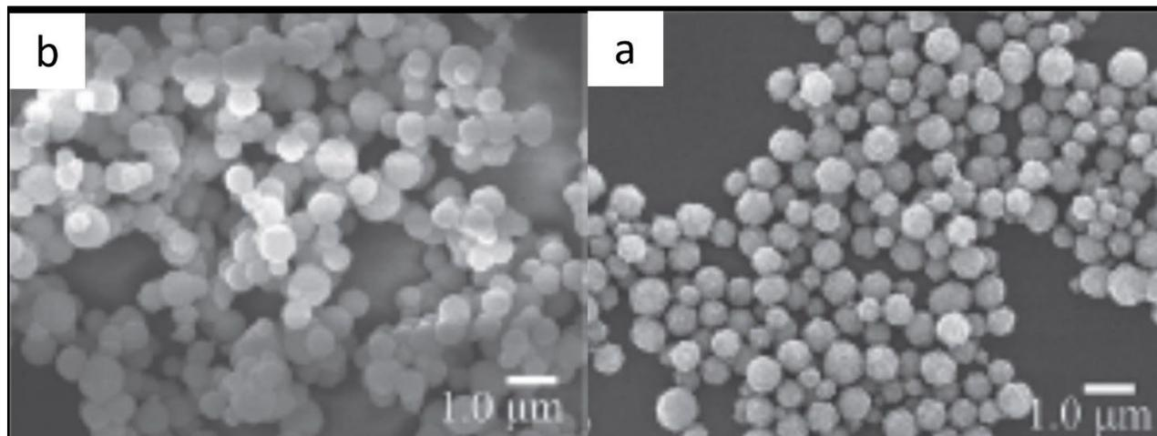
Figure 1. SEM images of titanium dioxide nanoparticles synthesized by homogeneous chemical precipitation at (a) 80°C and (b) 100°C [1].
