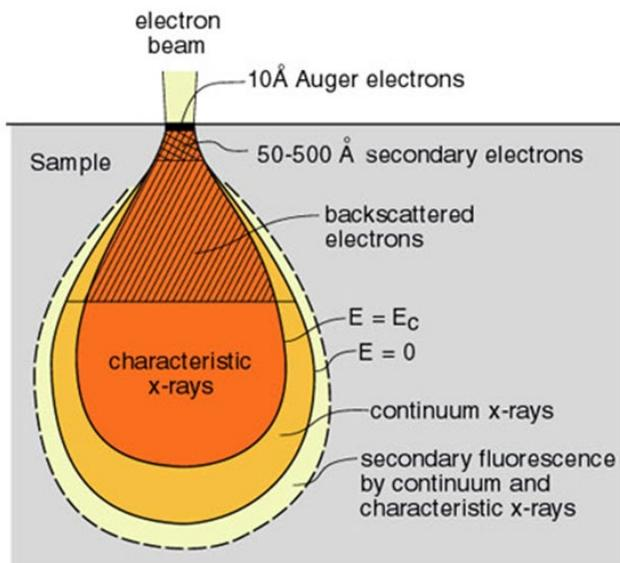
Figure 8 – Depth of penetration of different phenomena resulting from the interaction of the electron beam with the sample.
