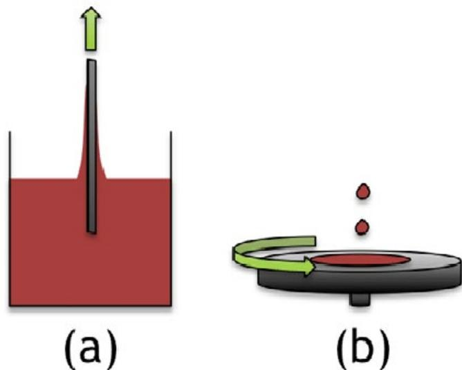
Figure 8 - Overview of coating methods: a) dip coating, b) spin coating.
