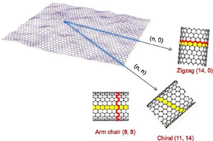
Figure 3: Types of carbon nanotubes based on chirality and angle [2].
