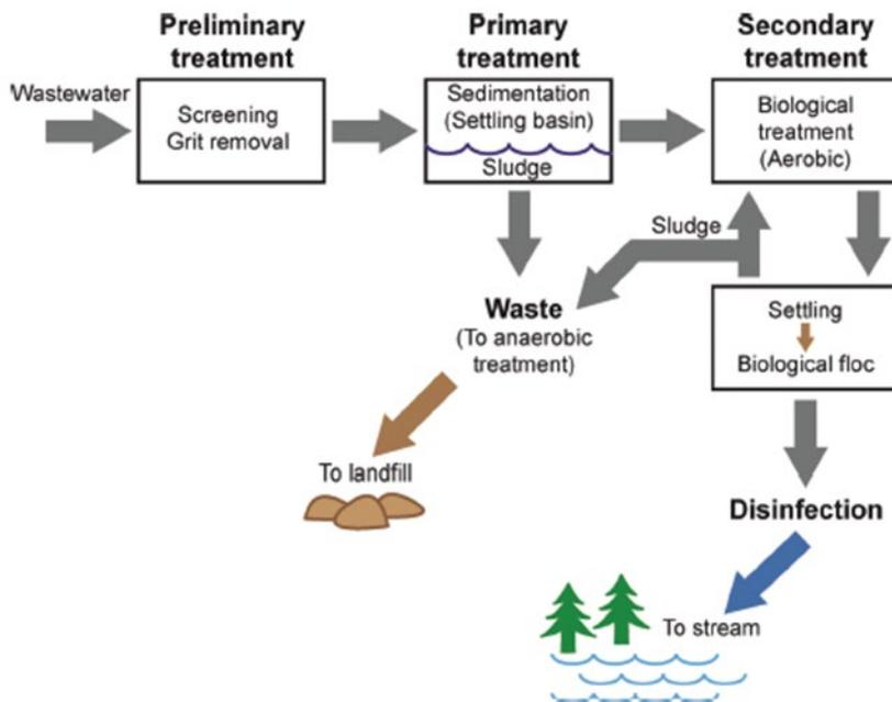
Figure 1 – Overview of the wastewater treatment process in a treatment plant[۲]
