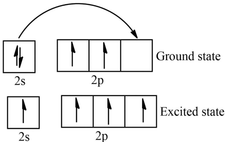
Figure 1: Electron configuration in the 2s and 2p levels of a carbon atom.
