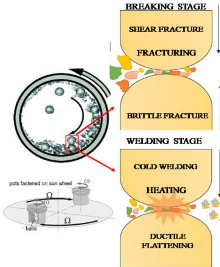
Figure 3 - Breaking and cold welding of particles during the milling process.
