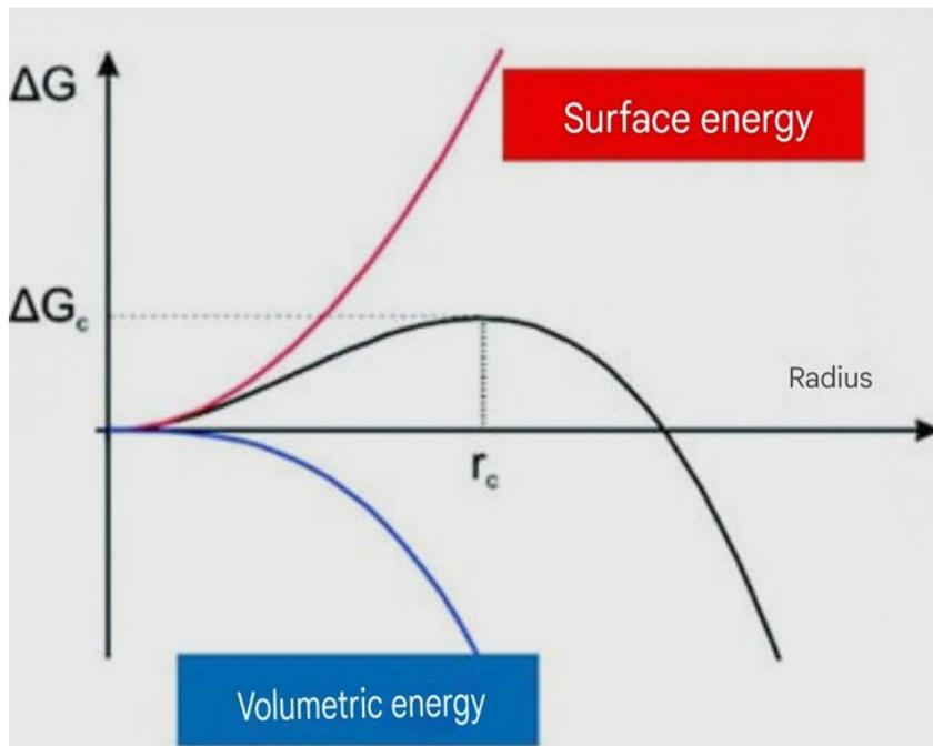
Figure 3: Changes in free energy based on the radius of the created nucleus [2].
