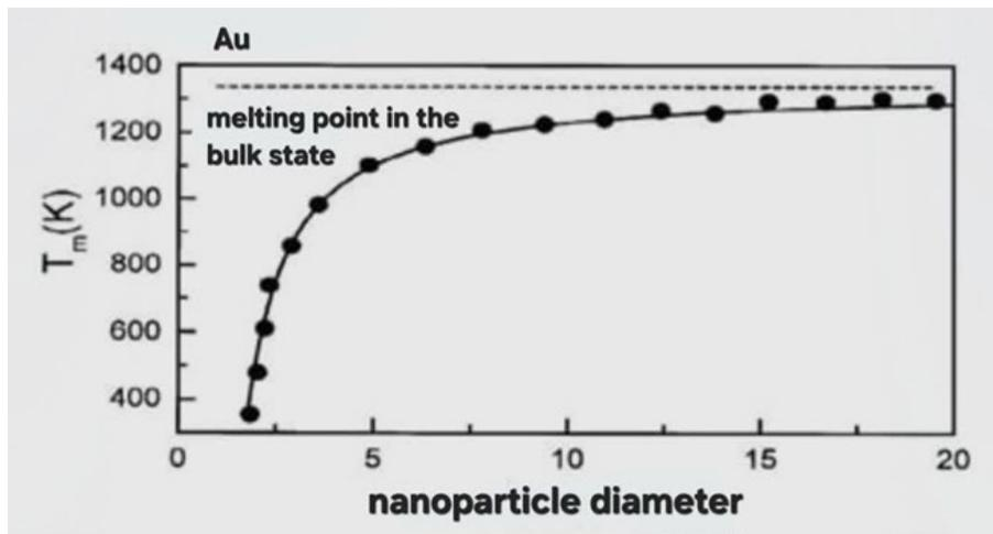
Figure 7: The effect of reducing nanoparticle size on the melting point of gold nanoparticles. The bulk melting point is shown as a dashed line; note the sizes [6].
