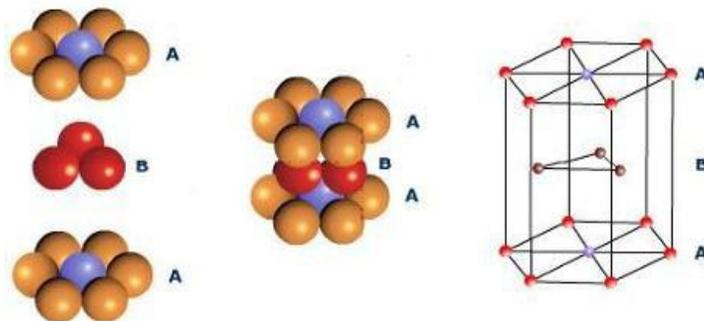
Figure 12: Showing the hexagonal close-packed lattice.
