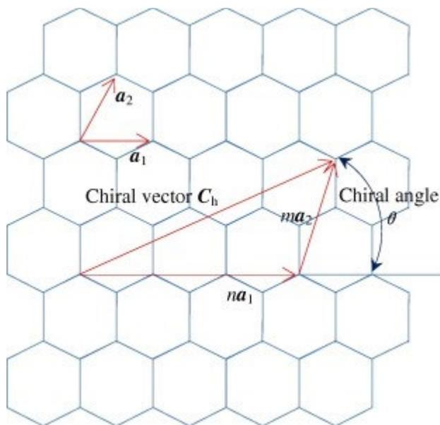
Figure5: Schematic diagram of the chiral vector and the chiral angle
