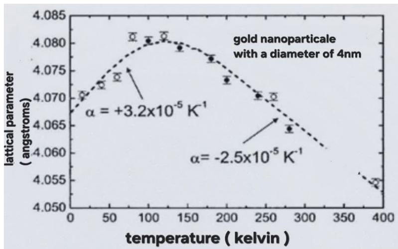
Figure 3: Changes in the lattice parameter and thermal expansion coefficient with temperature in gold nanoparticles [3].
