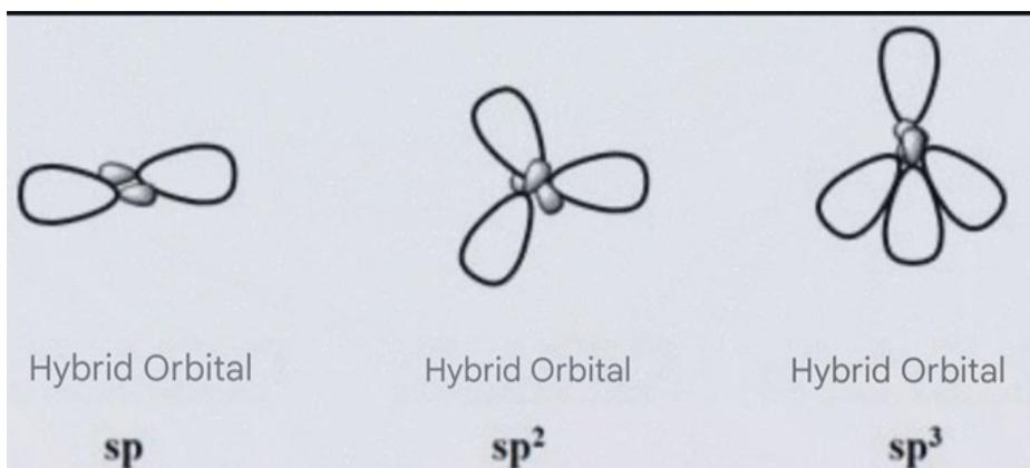
Figure 2: Diagram showing the different types of hybrids with varying bond angles.
