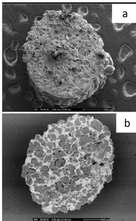
Figure 7 – (a) SE and (b) BSE images of the cross-section of a particle. SE is suitable for topographical and morphological imaging, while BSE is ideal for phase distribution contrast.
