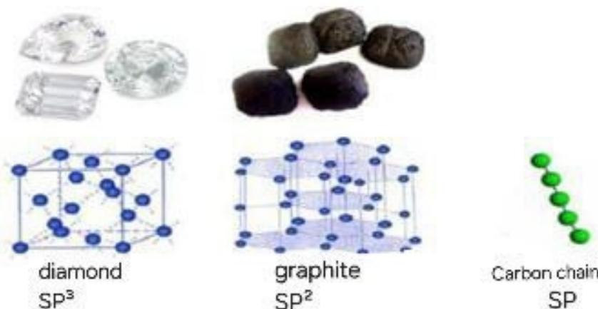
Figure 3: unit cells of one-dimensional, two-dimensional, and three-dimensional carbon compounds.
