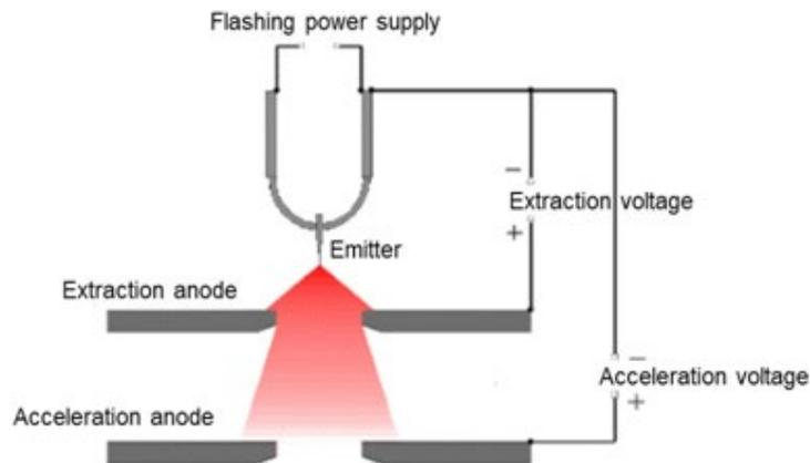
Figure 2 - field-emission electron gun: Electron Emission from the Metal Tip and Guidance by the Extractor Anode, Followed by Acceleration Using the Accelerator Anode
