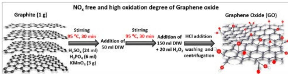
Figure 11: Steps of the modified Hummers method for synthesizing graphene oxide and reduced graphene oxide.
