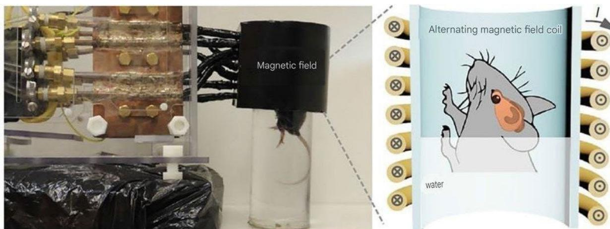
Figure 7 – Laboratory image of the drug delivery system using magnetic nanoparticles under a magnetic field and a diagram of a laboratory mouse placed in a coil of alternating magnetic field
