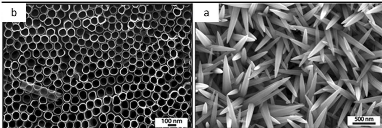
Figure 7: Images of one-dimensional nanostructures: (a) Titanium oxide nanotubes, (b) Zinc oxide nanorods.
