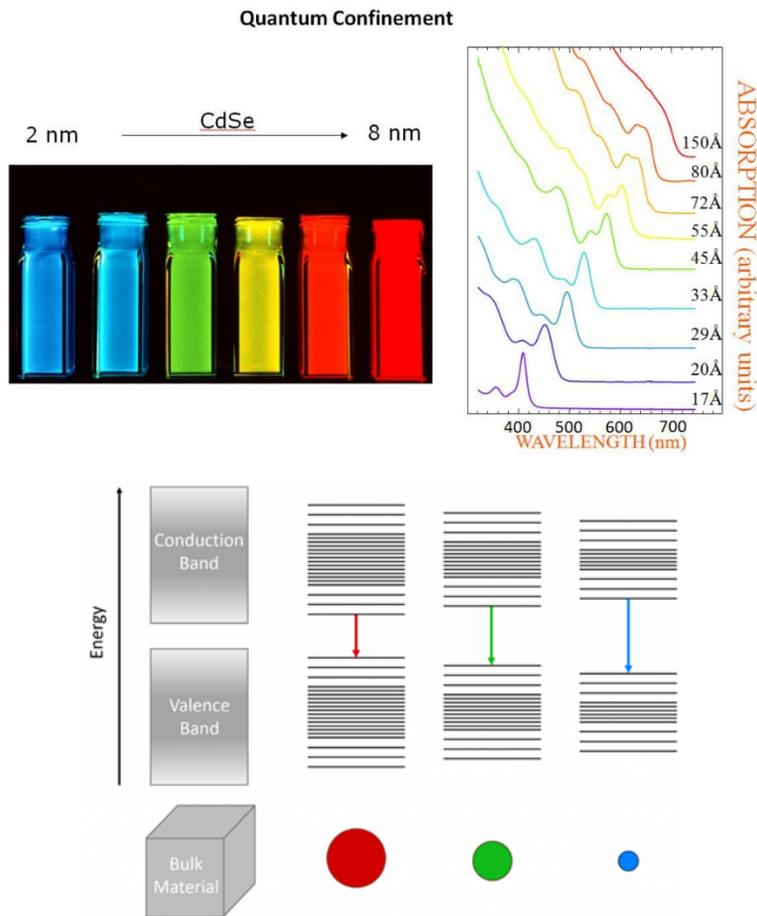
**Figure 2:** Top: Colors and absorption spectra of CdSe nanoparticles of different sizes. Bottom: The relationship between the electronic structure of quantum dots and their color at different sizes."
