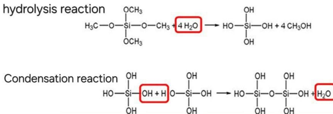
Figure 6 - Schematic representation of hydrolysis and condensation reactions for nanoparticle synthesis.
