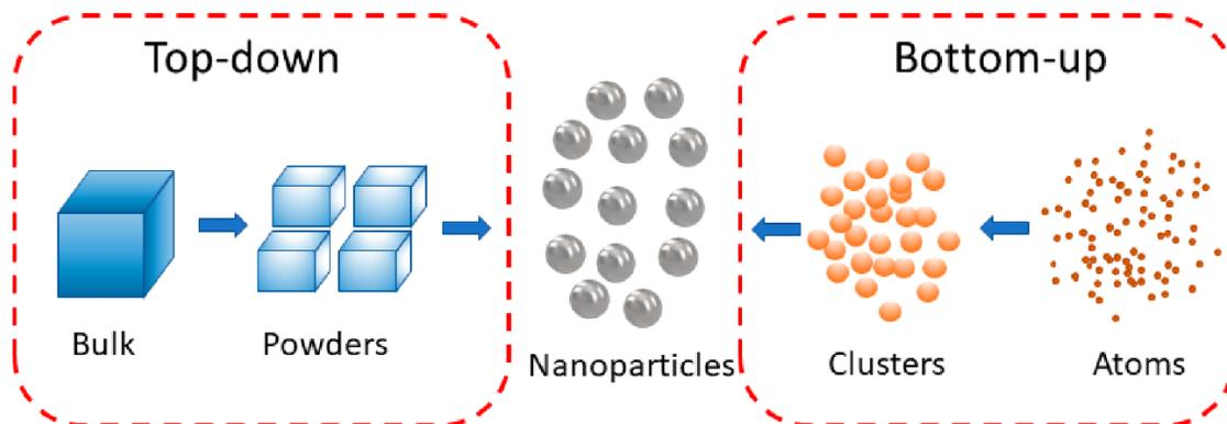
Figure 4- Diagram of Top-Down and Bottom-Up Approaches to Nanomaterials Production
