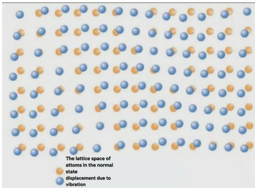
Figure 6: Schematic of atomic vibrations in a material due to atomic oscillations caused by heat application [1].
