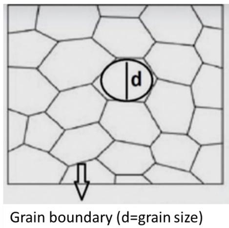
Figure 6: A polycrystalline material, with grain boundaries shown inside the square. The approximate size of a grain is the diameter of the hypothetical circle within it.
