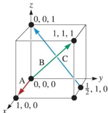
Figure 13: Showing some Miller directions in a cubic lattice.
