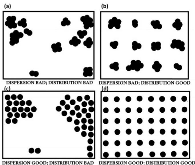
Figure 4: The concept of distribution and dispersion of reinforcing components in the matrix phase.
