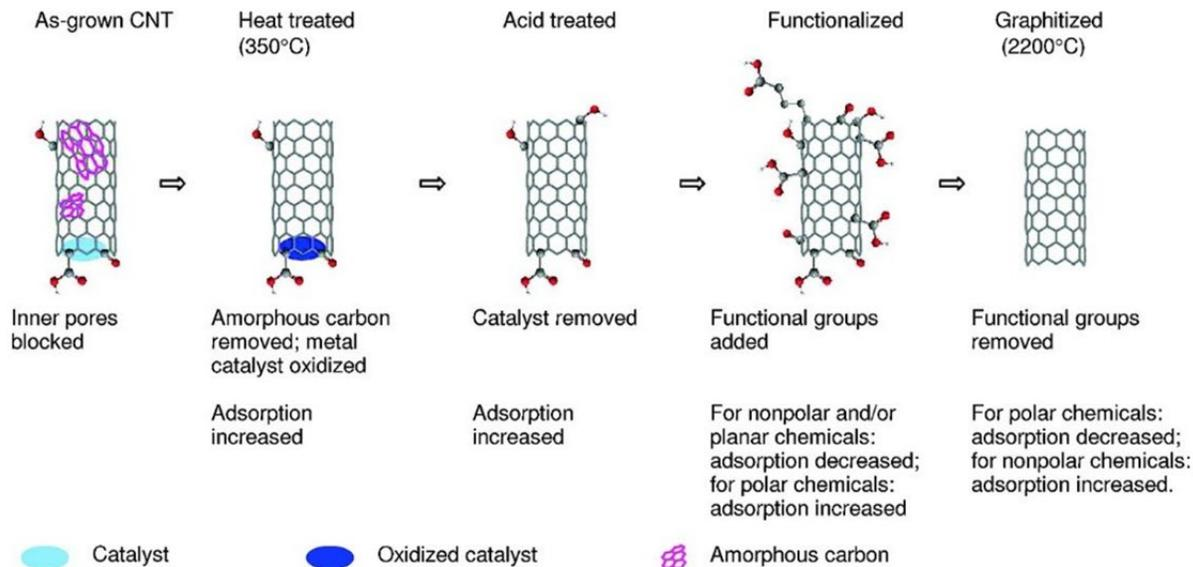
Figure1: The effect of various treatments and functionalization of nanotubes on their absorption
