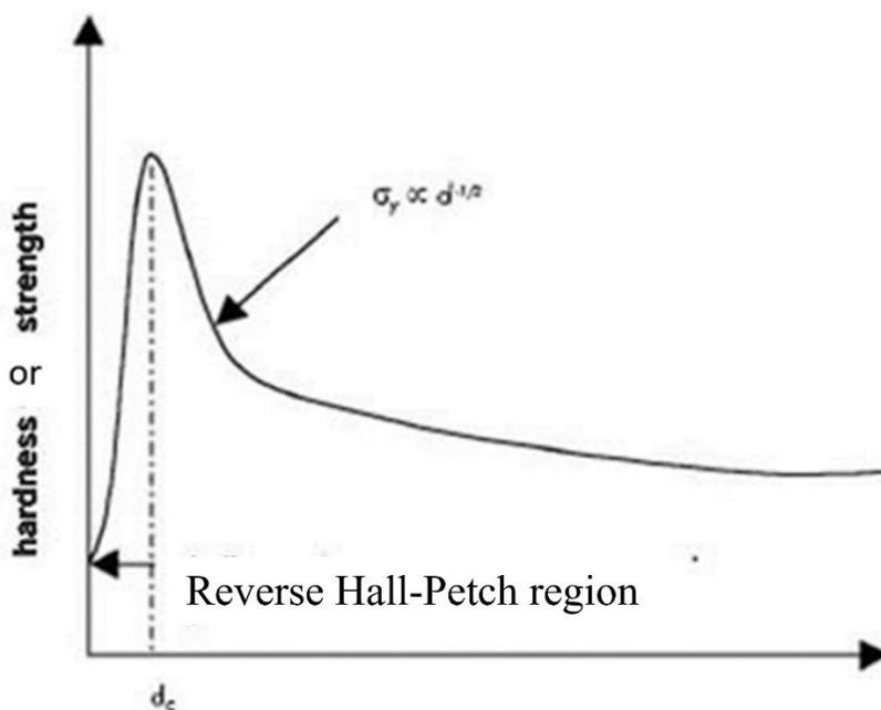
Figure 8: The graph illustrates the changes in material strength or hardness with variations in grain size.
