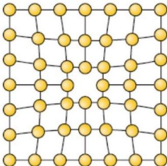
Figure 2: Representation of a vacancy defect in a crystal structure.
