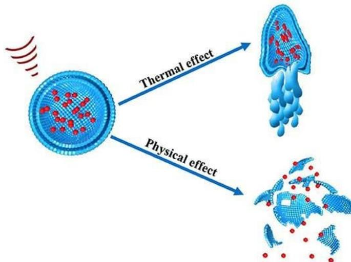
Figure 10 - A schematic of the thermal and physical effects of ultrasound waves in drug delivery systems[12].
