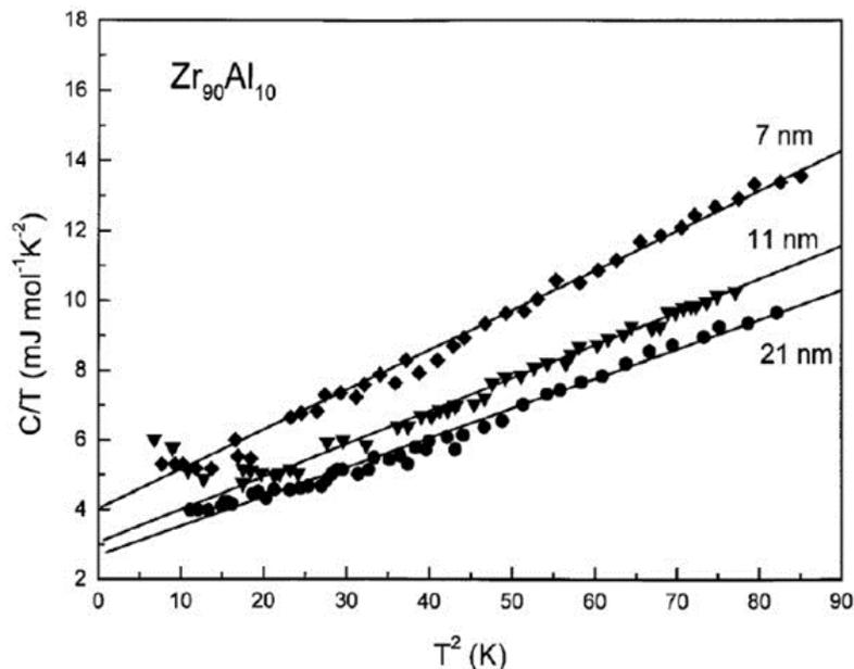
Figure 5: Impact of temperature on the specific heat capacity in ceramic nanoparticles of different sizes [4].
