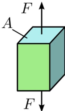
Figure 1: Stress caused by applying force to a surface.
