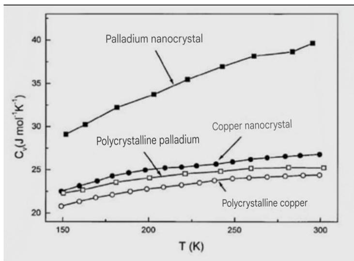
Figure 4: Impact of temperature on the specific heat capacity in nanocrystals and polycrystals (bulk) for palladium and copper [4].
