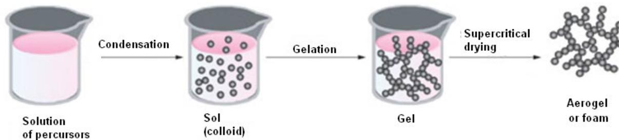
Figure 1 - Overview of different stages in the sol-gel reaction.
