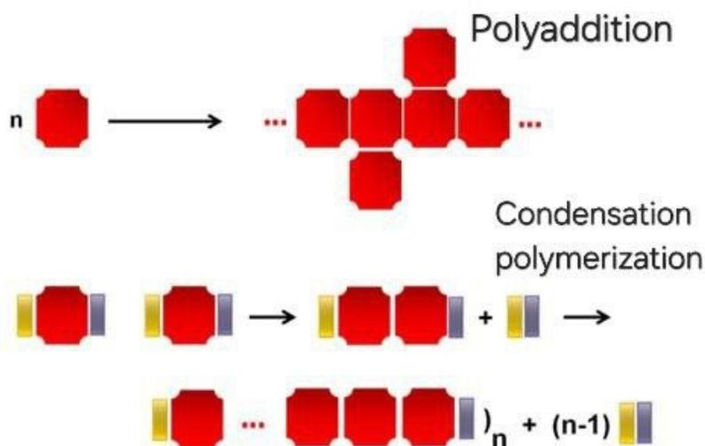
Figure 5 - Schematic representation of different polymerization processes.
