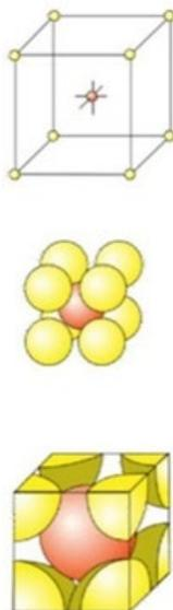
Figure 8: Schematic representation of a body-centered cubic lattice.
